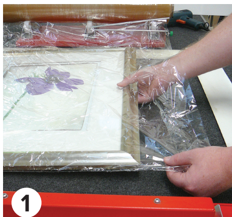
1 Slide frame between film layers and to left
