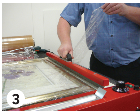
3 Seal and cut film to front
