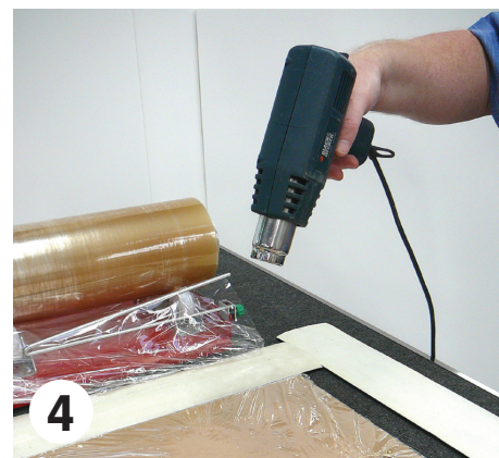
4 Apply heat to film on back of frame
