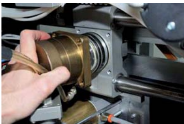
Lubricate and reinstall the cylinder.
