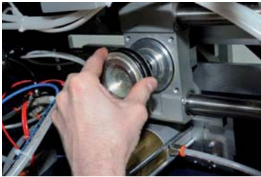
Lubricate and reinstall the piston.
