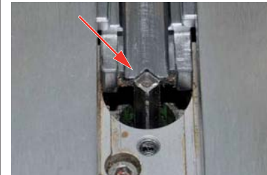
NB: align the hammer with the high part pointing towards the magazine.
