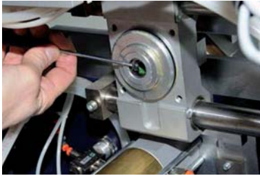
Replace the internal flange seal.
