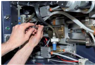
Remove the screws which hold the pneumatic cylinder in place.
