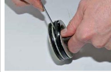
Replace both piston seals. If the hammer is worn out, proceed to replace the whole piston.
