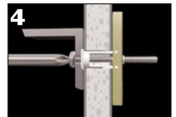
Place item over flange. Insert M5 bolt and tighten until snug against item, then stop. Use M5 machine screw or bolt locally to match thread in metal channel.
