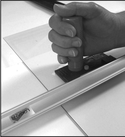
Figure H-4: Pull the glass cutter back, scoring the surface of the glass.
