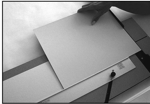
Figure L-4: Place the mat blank against the squaring arm and the mat guide.
