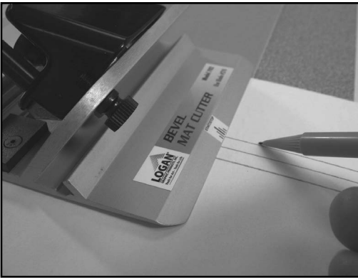
Figure S-6: Align the start/stop indicator line with the top of the outermost rectangle.
