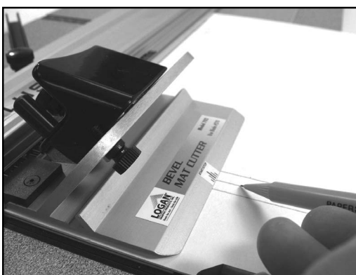
Figure S-4: Cut until you reach the bottom of the middle rectangle.
