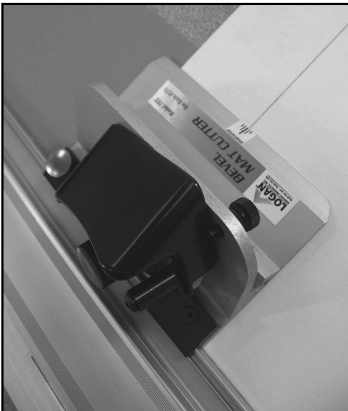
Figure L-7: Align the start / stop indicator line with the intersecting pencil line.
