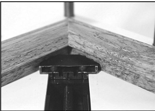
Figure J-3: Adjust the moulding sections in the clamp so the top corner is square.
