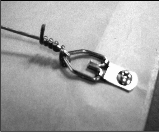
Figure CC-3: Coil the wire around itself several times.
