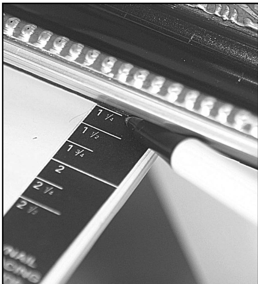
Figure J-4: Measure the width of the moulding using the set block scale on the clamp.
