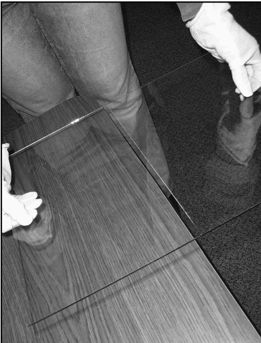
Figure H-5: Align the score along the edge of the table and snap the glass cleanly along the score.
