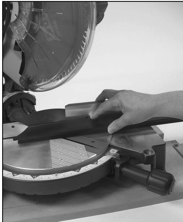
Figure E-2: Place the stick of moulding against the saw fence finished side up with the rabbet facing toward you.
