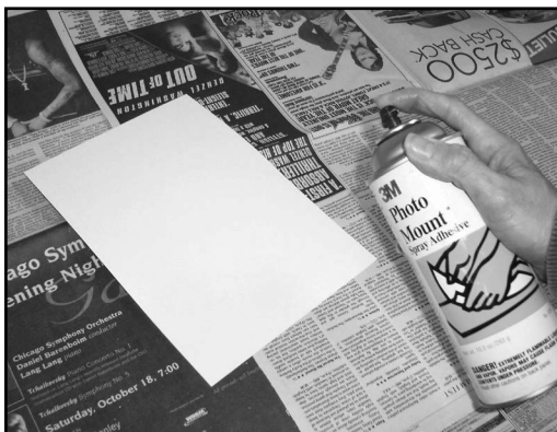
Figure U-1: With spray mounting, the adhesive is sprayed from 8 to 12 inches away in a sweeping motion.
