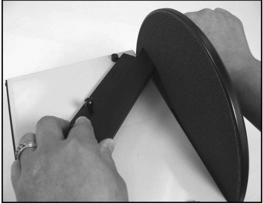
Figure F-3: Press the miter face against the disc.
