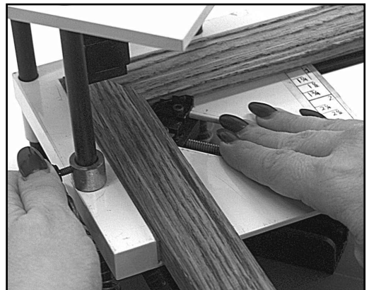
Figure J-1: Lock the clamp down using the clamp locking collar.
