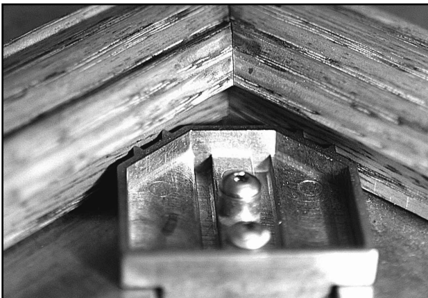
Figure I-5: Adjust the joint so the two miters are aligned.
