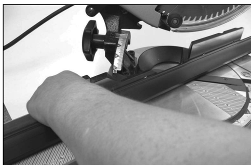
Figure E-8: Place the second stick of moulding against the fence so the finished side is up and the rabbet facing toward you.
