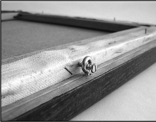
Figure X-3: A screw eye set into the back of the frame provides a loop through which a regular screw can be inserted.
