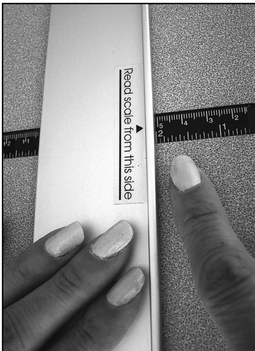
Figure L-2: Set the mat guide on the scale for the border you want to cut.
