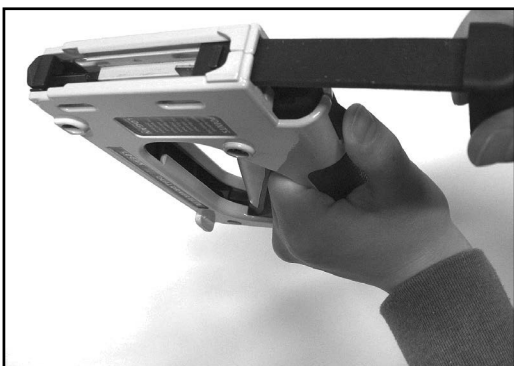
Figure Z-11: Slide back the point loading cover.
