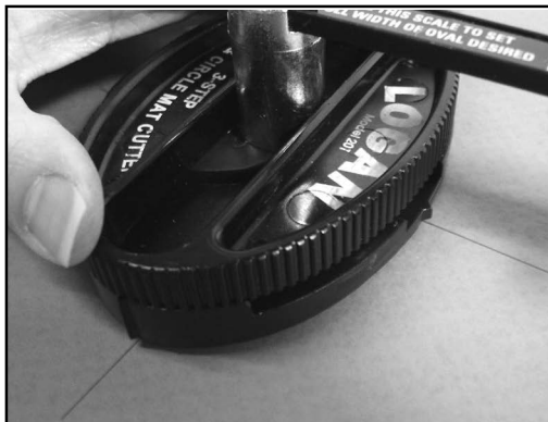
Figure P-4: Align the pointers on each side of the base with the arms of the plus sign.
