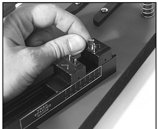
Figure J-9: Remove the V-nail block cartridge and load V-nails onto the V-nail blocks.
