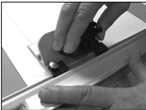
Figure L-10: Cut the mat, applying firm downward pressure on the cutting head as you pull it back.
