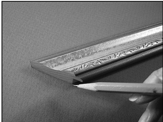
Figure D-2: The 45-degree cut at the end of each section is called the "miter."
