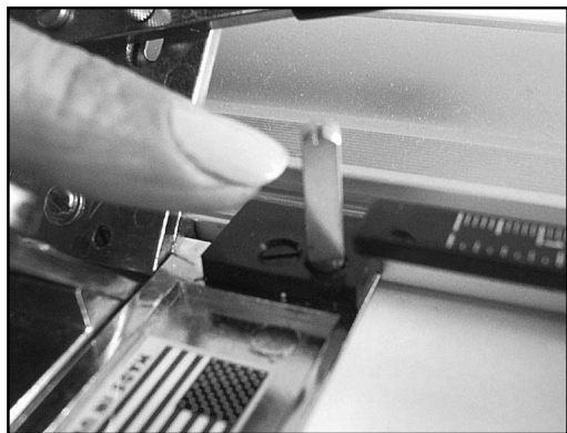
Figure Q-2: To adjust the stopping point of the mat cutter, adjust the eccentric post.
