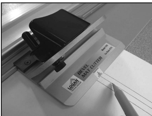
Figure S-3: Align the start and stop indicator with the top of the middle rectangle.
