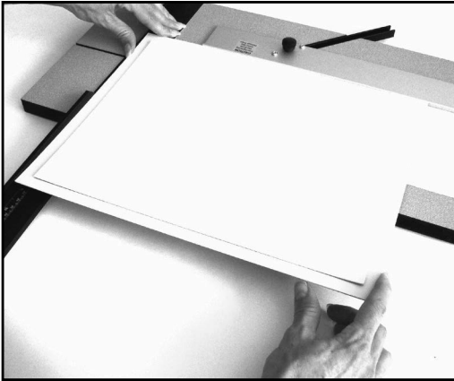
Figure N-4: Place the stack of two mats under the guiderail and firmly against the mat guide.
