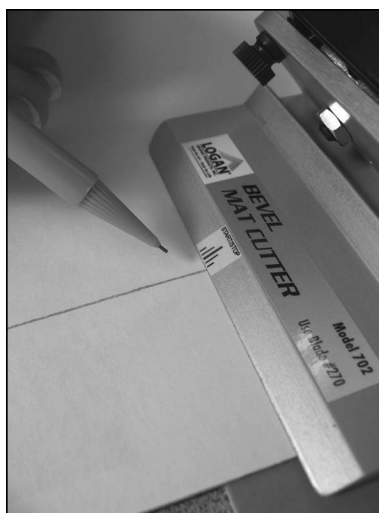
Figure M-3: To eliminate overcuts and undercuts, move the start and stop indicator line in proper relation to the pencil line.
