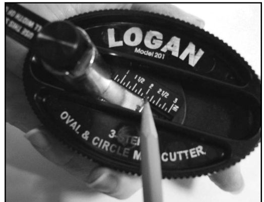
Figure P-1: A cam-shaped plate with an adjustable mid-point allows for the setting of different ellipses.
