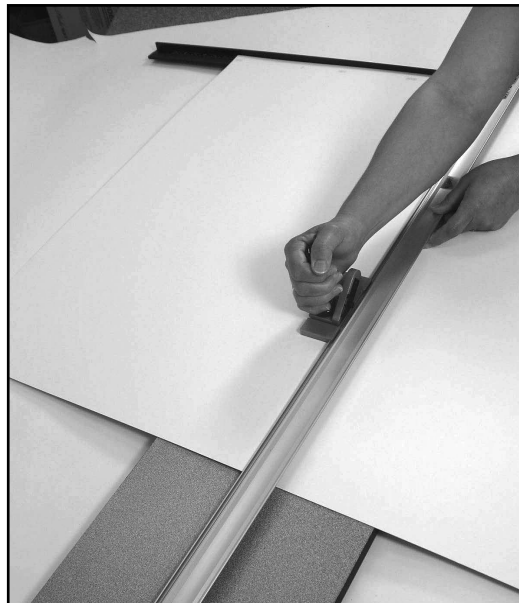
Figure G-6: Pull back toward you, cutting the sheet.
