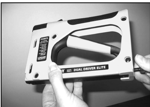
Figure Z-13: Adjust the drive strength.
