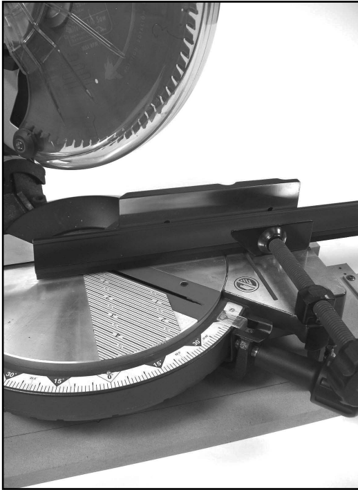
Figure E-3: Move the moulding just past the slot in the saw fence so a 45-degree cut can be made at the end of the stick.
