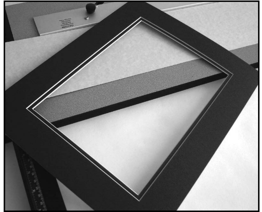
Figure N-5: Cut the undermat. The result is a perfectly aligned double mat.
