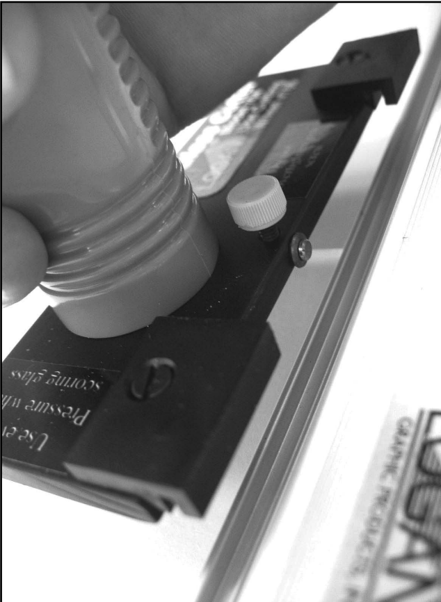
Figure H-3: Hook the glass cutter onto outermost lip of the guide rail.
