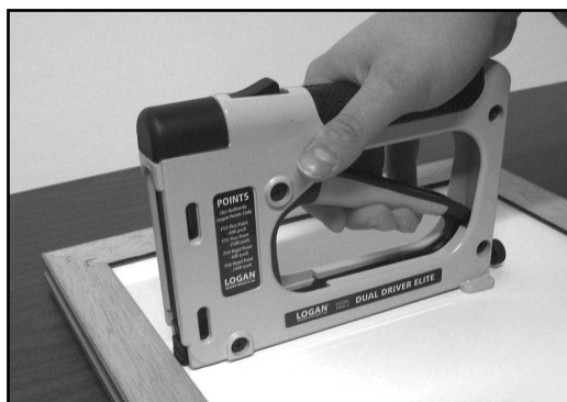
Figure Z-14: Place the nose of the driver against the inside of the frame rabbet.
