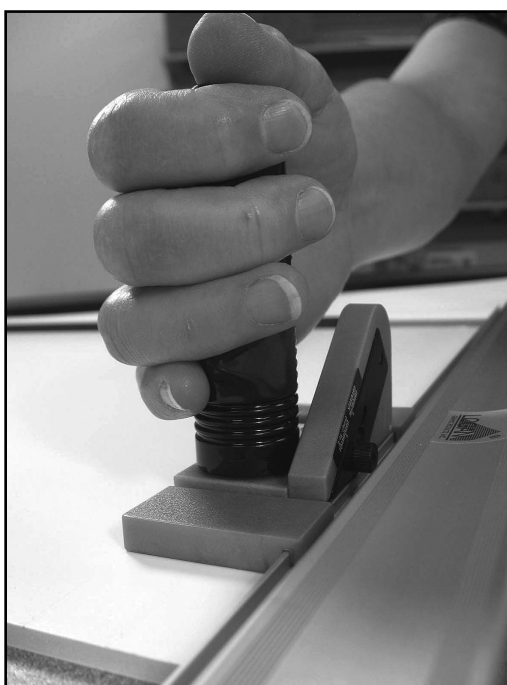
Figure T-1: Cut a sheet of 1/8" thick foamboard into narrow strips.
