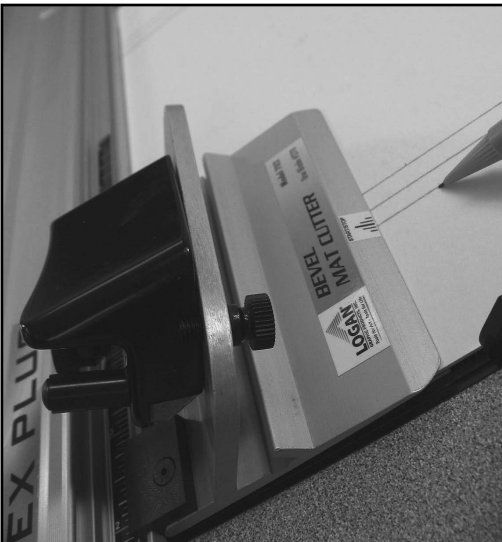
Figure S-7: Cut until you reach the bottom of the outermost rectangle.
