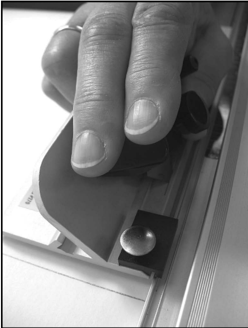
Figure L-6: The plastic guides clip over the outer lip of the guide rail.
