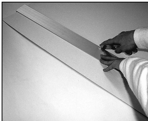
Figure G-7: To size outside a mat cutter, score repeatedly with your mat knife along the straightedge.
