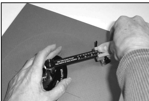
Figure P-9: During the final rotations exert moderate downward pressure with your thumb on top of the cutting head.
