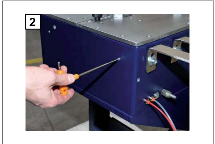
2. Remove the grub screws from the machine body.
